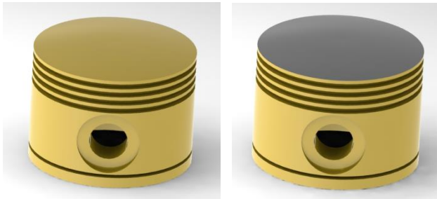
Fig 3: 3D model of piston without and with TBC Coating
